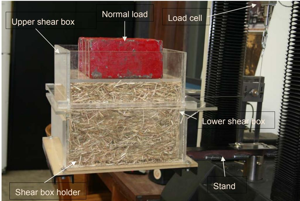
Figure 1. Direct shear cell with biomass before shearing.
