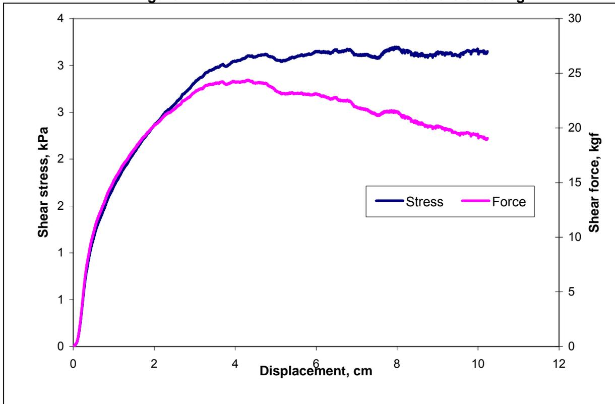
Figure 2. Typical shear stress and force curves during shear tests of chopped biomass
